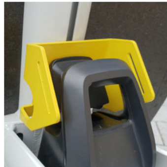
2.2 Click the battery into the bike and adjust the lock properly if necessary.
