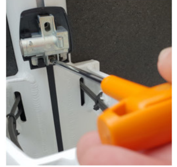
1.4 Unscrew the two Inbus screws.
