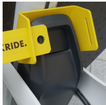
2.5 Slide the pin into the bracket and lock it with a disc or padlock.
