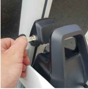
1.1 Remove the battery from the bicycle.
