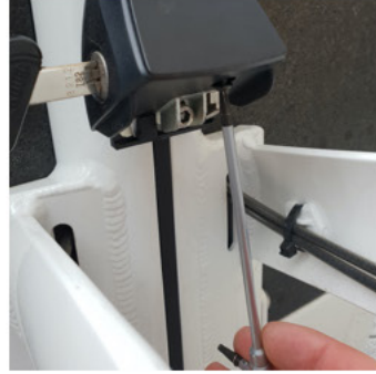
1.2 Unscrew the lock cap at the bottom with a Torx screwdriver.
