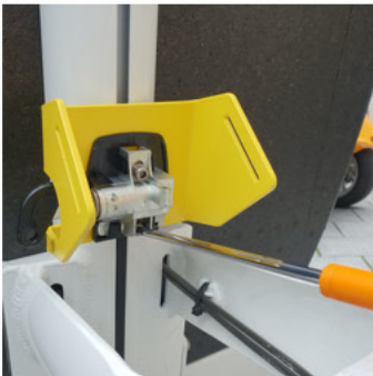
2.1 Install the Lockride bracket, but do not fully tighten the bolts yet.
