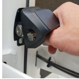
1.3 Unclip the lock cap by gently bending it open to the sides.
